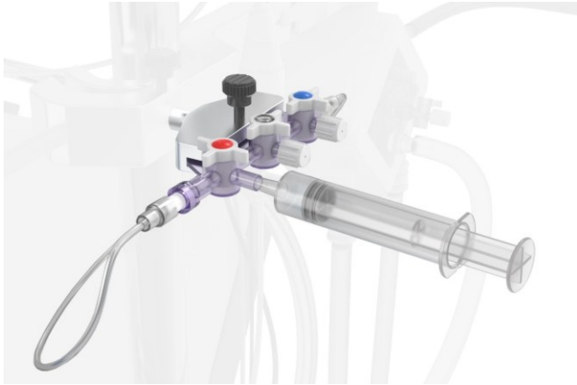
Figure 20 De-air the sample line by aspirating with a syringe. Ensure that the red valve is in the orientation indicated.
